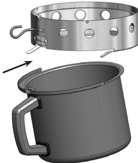
Ensure slot in the base engages the clip in the air vent as illustrated.
